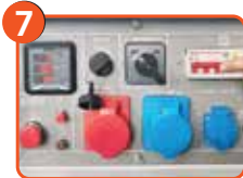
7 TURN ON THE CIRCUIT BREAKER.
